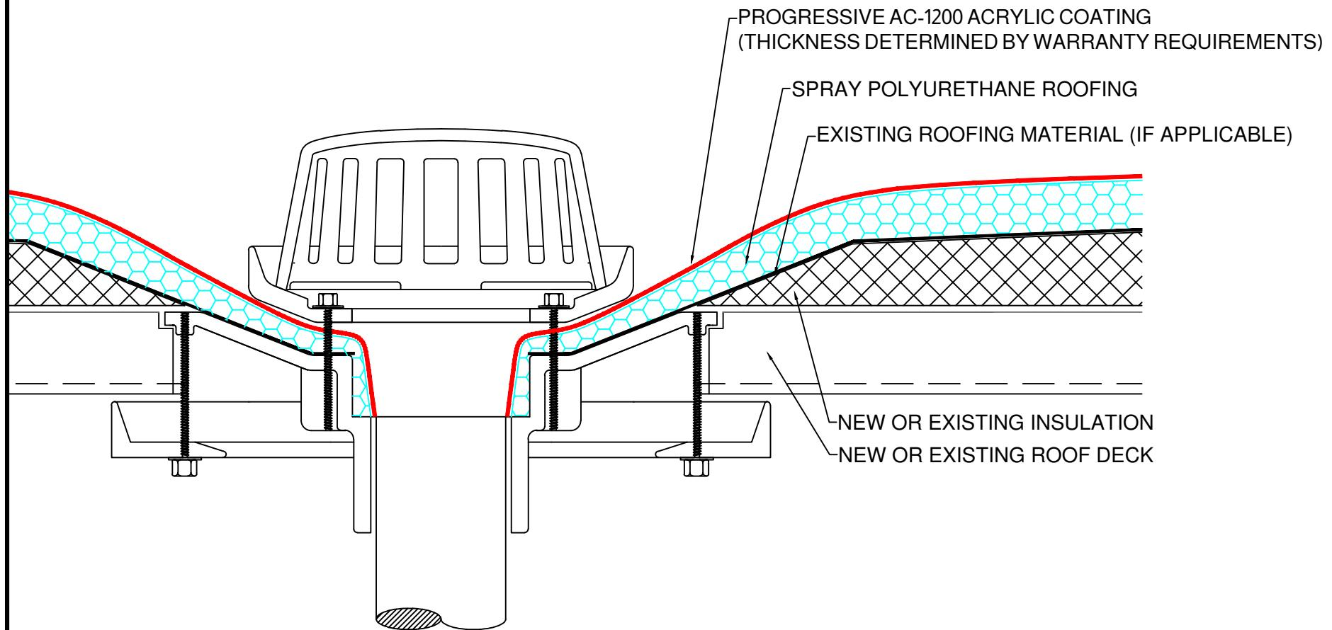
Detail: Roof Drain Detail
